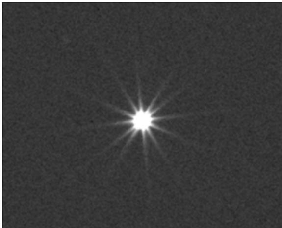
FIGURE 2.4.12. THE MASK WITH TRIANGLES CREATES DIFFRACTION SPIKES, WHICH MAKES IT EASIER TO TELL WHEN THE TWO IMAGES ARE MERGED. THE SPIKES WILL ALL POINT TO THE SAME PLACE WHEN THE IMAGES OVERLAP.
