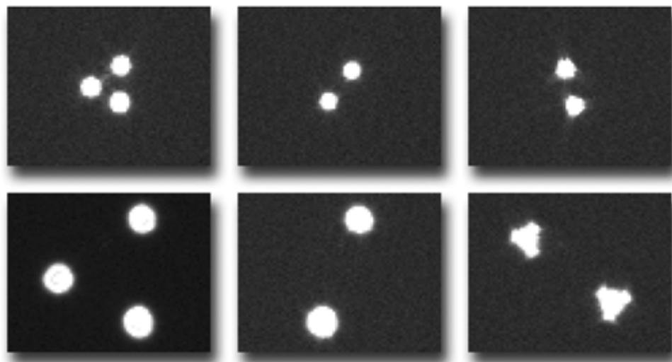
FIGURE 2.4.II. RESULTS OF USING THE THREE MASKS. LEFT: THREE ROUND HOLES. MIDDLE: TWO ROUND HOLES. RIGHT: TWO TRIANGLES. OUT OF FOCUS AT THE BOTTOM; IMPROVING FOCUS AS YOU MOVE UPWARD.
