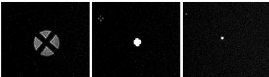
FIGURE 2.4.2. LEFT: STAR WELL OUT OF FOCUS, SHOWING SHADOW OF MASKING TAPE. CENTER: CLOSER TO FOCUS, SHADOW IS LESS PROMINENT. RIGHT: CLOSE TO FOCUS, SHADOW DISAPPEARS.
